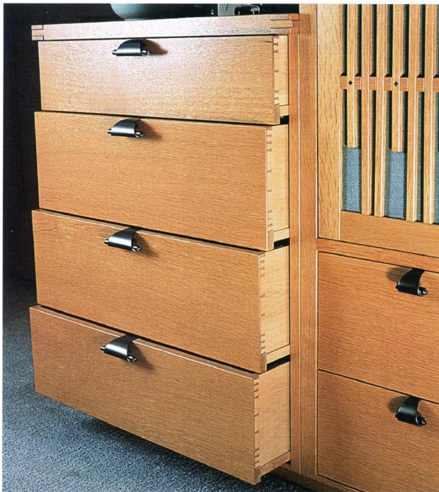
HAND-CUT JOINTS AND HANDMADE PULLS FROM INDIA. All of the drawers have variably spaced, hand-cut dovetails. The author sandblasted the shiny original finish on the pulls, then patinated them antique brown.
